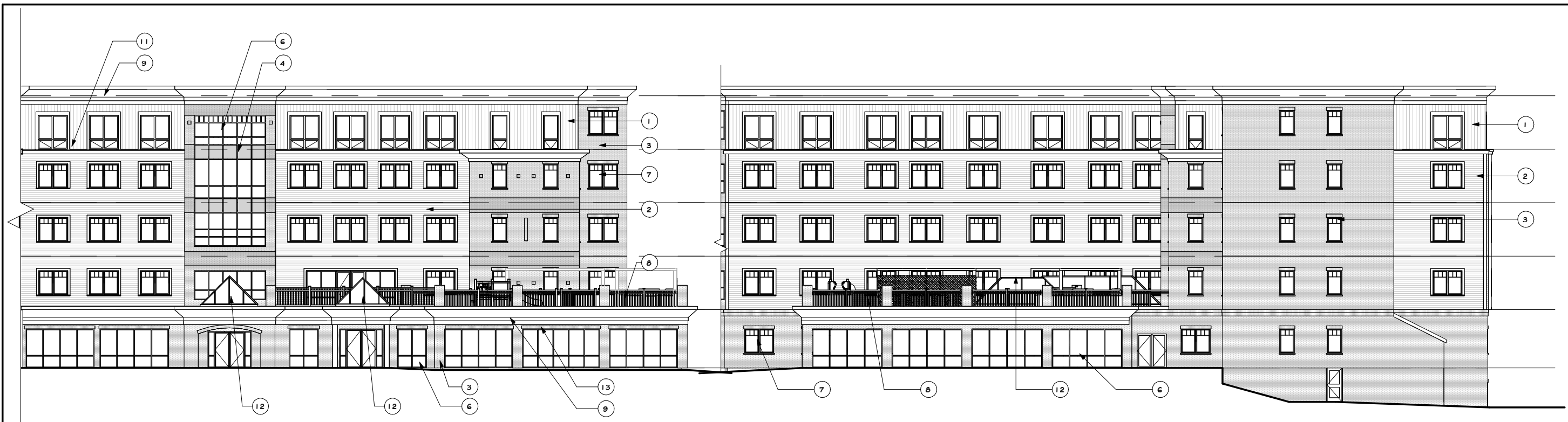
1 FAMILY BUILDING - NORTH ELEVATION A 3/64" = 1'-0"
