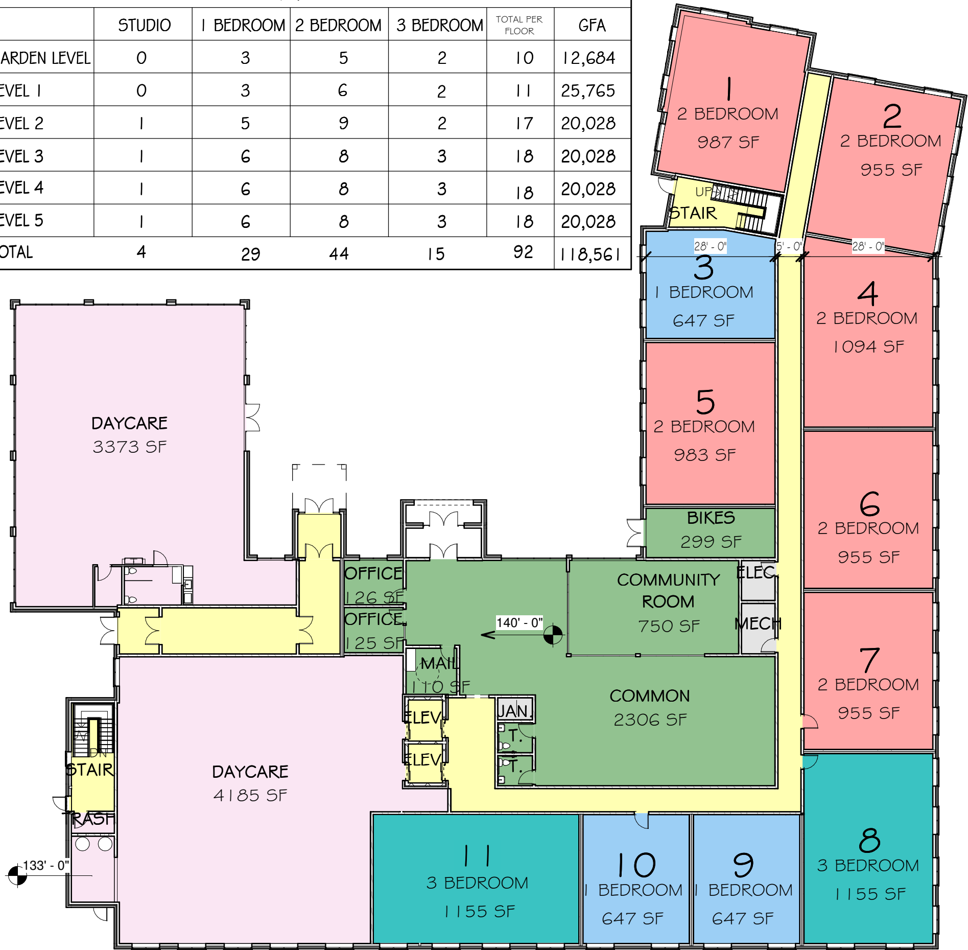
① LEVEL 1 FLOOR PLAN 3/64" = 1'-0"
